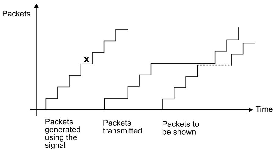
In the figure, we can see that the excessive delay experienced by packet x forces the reproduction to stop until it arrives. One way of minimising this effect is to buffer the information received so that reproduction begins with a certain amount of delay, and this is decided beforehand by estimating the average delay that the packets may experience.
