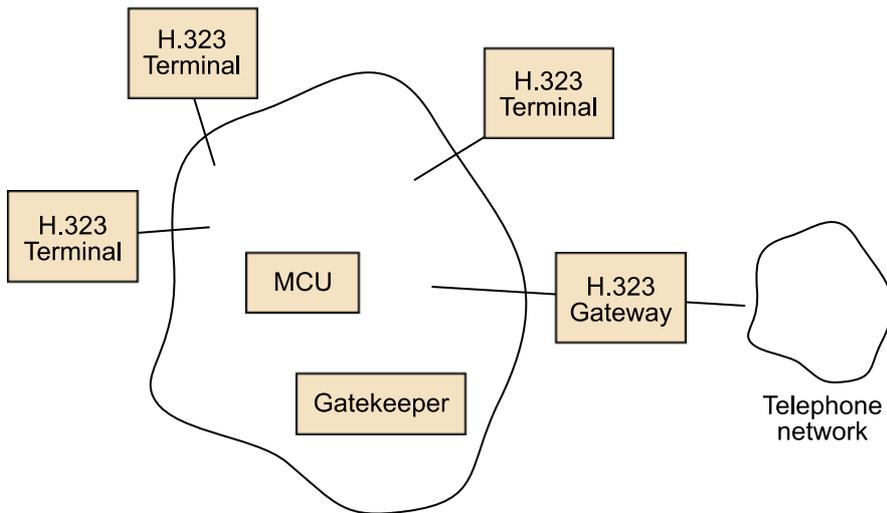
We can distinguish between four types of components which, when inserted into the Internet, provide point-to-point and point-to-multipoint multimedia communications:
