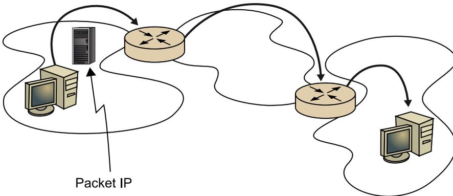
Routing is done using routing tables that contain a limited but sufficient quantity of information to allow connections between all the networks on the Internet. Each device connected to an IP network requires a routing table.
