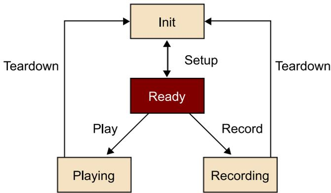
The initial state is *Init*. When a SETUP is sent and a positive response is received, the client and the server pass to *Ready*. From here, they pass to *Playing* or *Recording* depending on whether a PLAY or a RECORD was sent (and a confirmation received). The PAUSE command returns the state to *Ready*, another PLAY or RECORD command will return the state to *Playing* or *Recording*. The TEARDOWN command always returns the state to *Init*.
