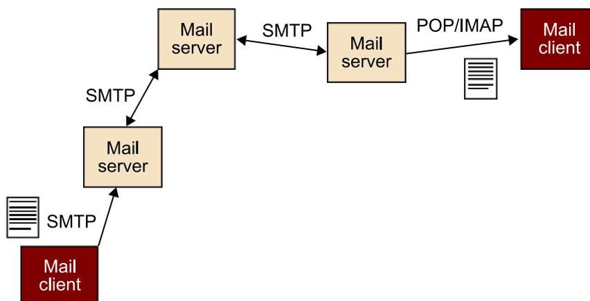
When we compose a message, it is stored in the server the e-mail client is connected to. The servers connect periodically and pass on messages that are then in turn retransmitted. This continues until they reach the domain of the destination user. The protocol which moves messages over
