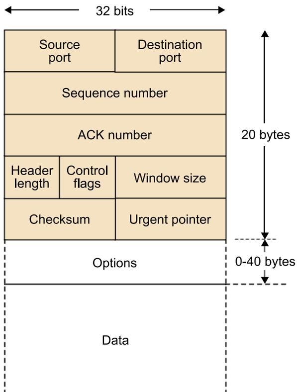
TCP packet headers have 9 fixed fields plus an option field usually used if options need to be specified:
