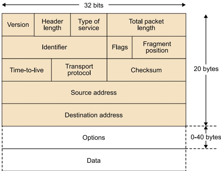
We can see that they have two parts: The header and the data being transported. IP packet headers have 12 fixed fields plus an option field usually used if options need to be specified:
